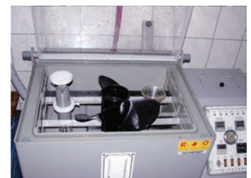
Salt Water Spray Testing
